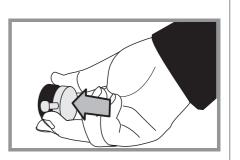
The grill has a special safety device with stops the flow of gas to the grill if the flame goes out. Turn the knob to the large flame symbol (). Press in the grill knob. This lets gas through to the burner. Keep holding the knob pressed in and press the igniter button or light with a match. Keep holding the button for about 10 seconds
